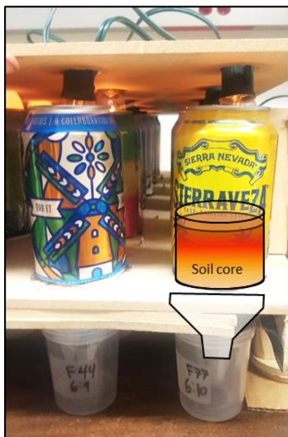
Fig. 4 (left) We built a custom Tullgren-funnel extractor, which uses light and aluminum casings around soil cores to create a heat gradient that forces mites to leave the soil and collect in sample vials below.
